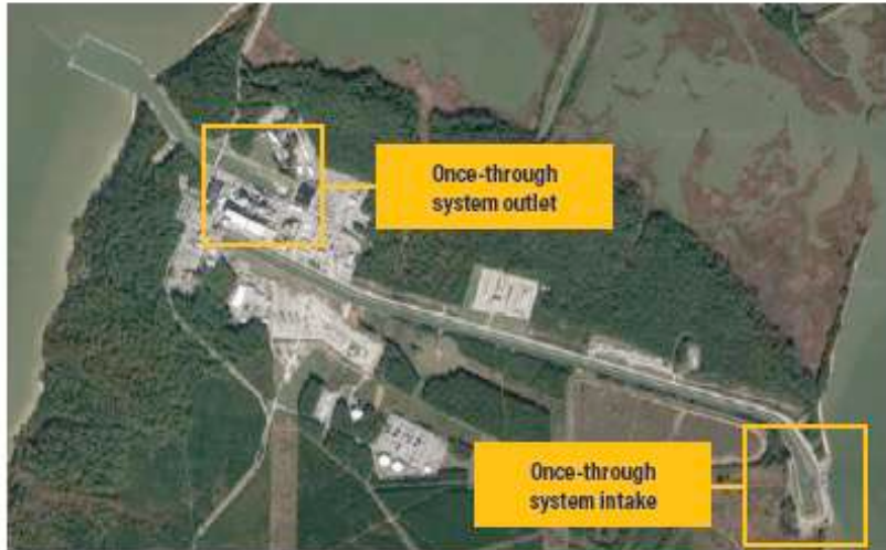
Figure 2 | Satellite Images of a Once-Through System
